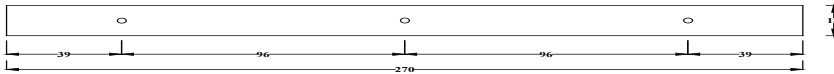
Fig. 2: Typical placement of dowel and screw centers in the L type corner joint.
