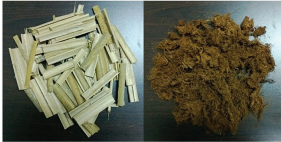
Fig. 1: The untreated bamboo chips and steam-exploded bamboo fibers (3.0/180).
